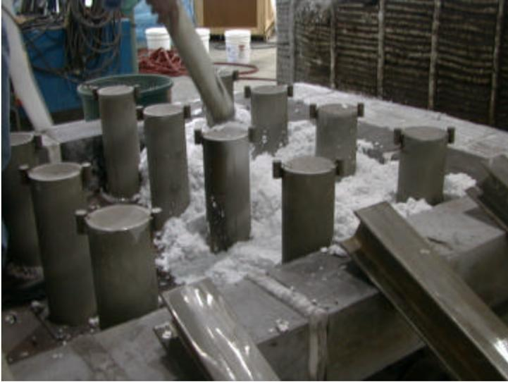
The Foamfrax Insulation was gunned into the car body tightly around the support piers and against the castable refractory perimeter.
